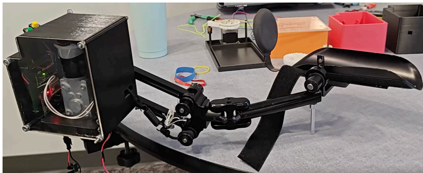
Figure 1: Tensioning device attached to JAECO MultiLink Mobile Arm Support
